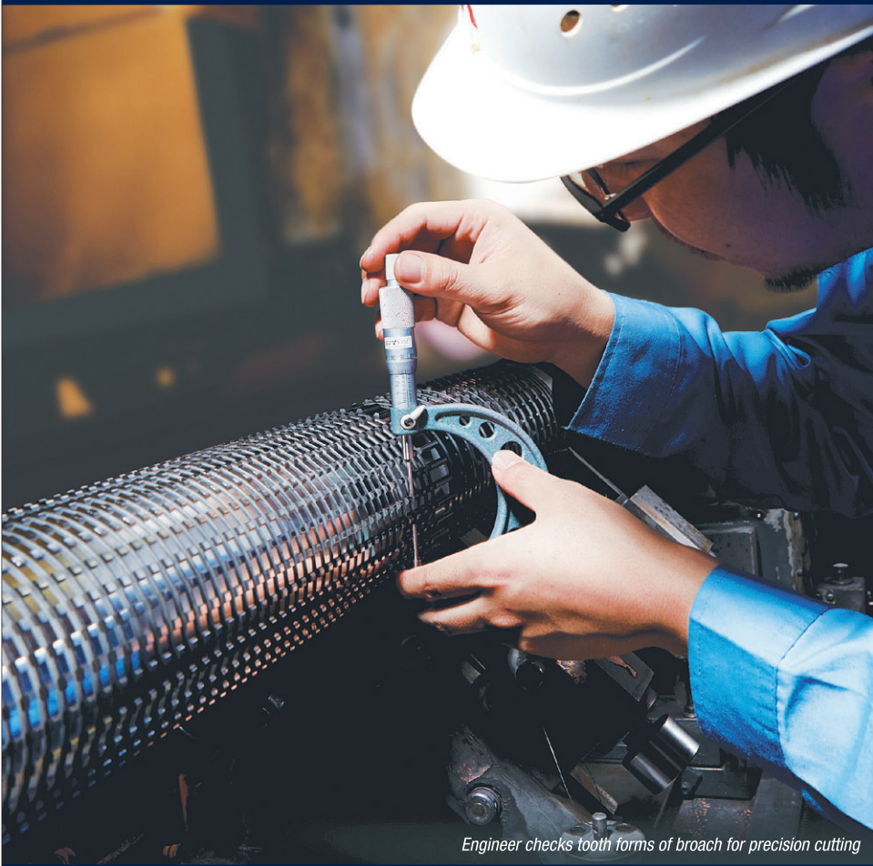
Engineer checks tooth forms of broach for precision cutting
