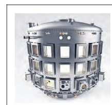
The ITER cryostat, designed to house superconducting magnets and deliver a super-cool fusion environment
