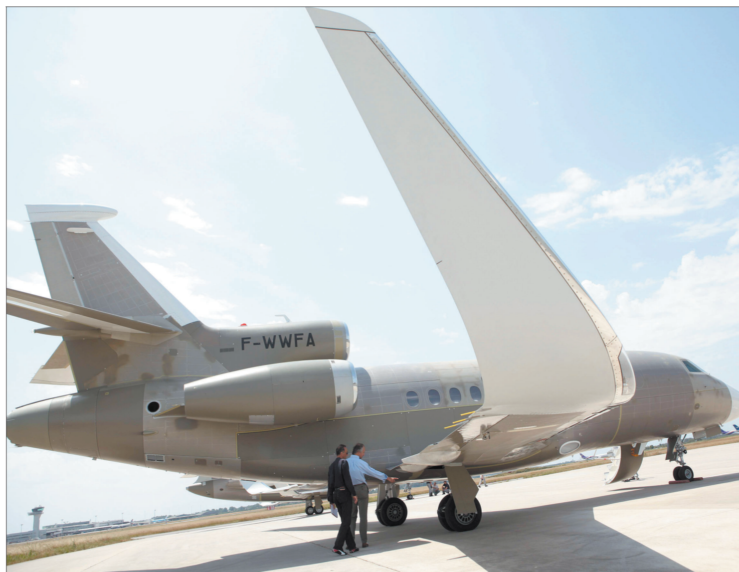
Fresh from the line: aerodynamic tweaks give the Falcon 900LX 5 per cent better fuel efficiency in the cruise
