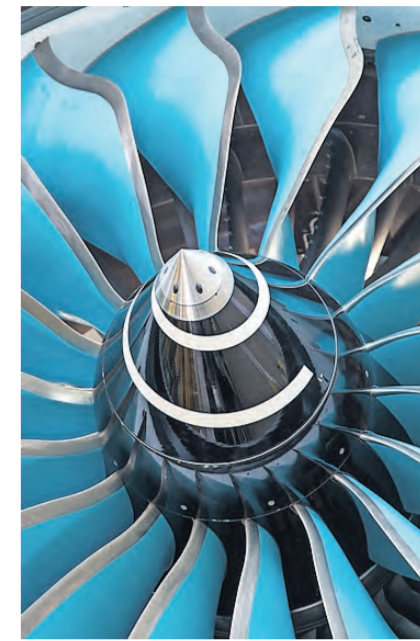
Big fan: a carbon and titanium engine
