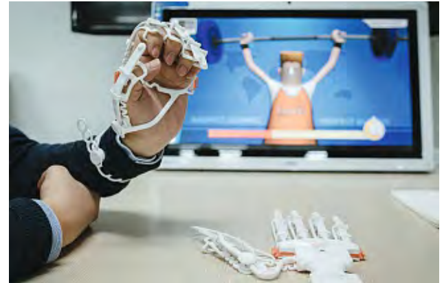
Gripping: Hoyoung Ban (right) with Neofect's 'glove' (also above). The device works with online games to help people recover from strokes
